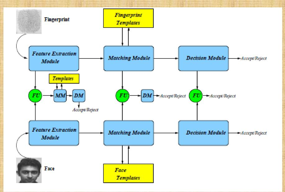
Level of Fusion in a bimodal biometric system FU: Fusion Module, MM: Matching Module, DM: Decision Module.
