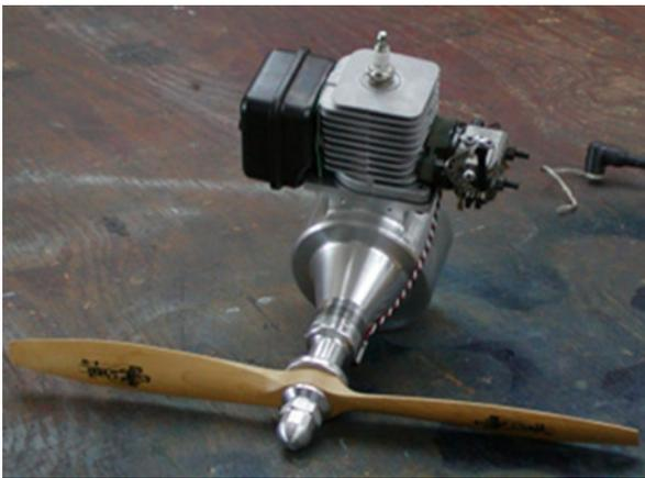
**Figure 3. 30cc Wiseman Mechanism Prototype Engine**
