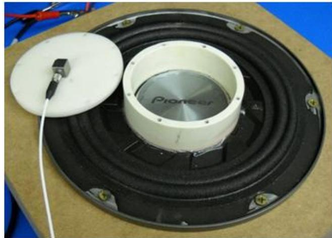
**Figure 4. Subwoofer Shaker-table Detail**
