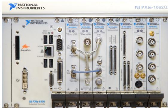
**Figure 7. National Instruments PXI-4462 Dynamic Signal Acquisition Device (the first module from the right) and PXIe-1062Q PXI Express Chassis**
