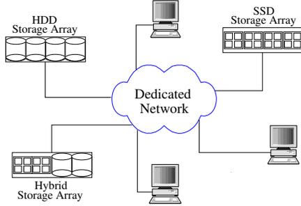
Fig. 1. Storage arrays connected with a dedicated network
